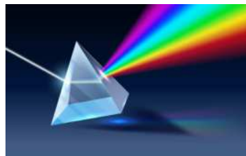
Figure 7.5: Dispersion of white light by a prism
