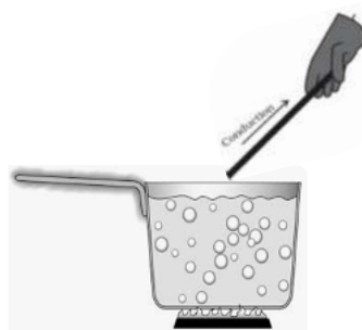
Figure 7.15: Heat transfer through metal stick by conduction
